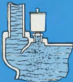
**ELIMINAIRE**<sup>®</sup>—A patented cost-saving feature. This built-in air eliminator is cast into the front section of all V<sub>1</sub> Series boilers to divert rising air bubbles into a tapping for connection to the expansion tank. No external device is required to separate air and water, reducing cost and installation time.
